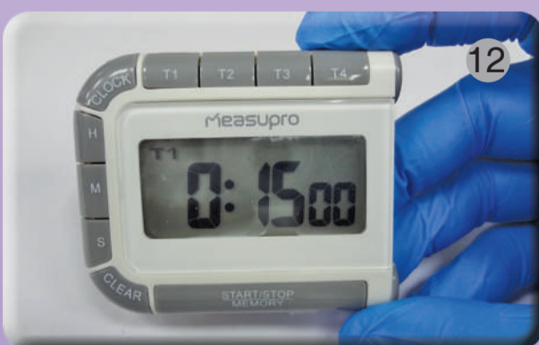
Read test results at 15 Minutes. Don't interpret after 25 Minutes.
