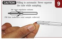
Hold the tube horizontally, and touch the tip of specimen transfer device to the blood. Capillary action will automatically draw the blood to the fill line(35µl) and stop.
